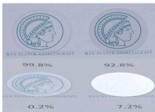
nanoAR (left) and reference (right): transmittance (top) and reflection (bottom).
